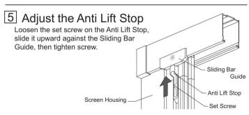
Note; in some cases the Anti Lift Stop may not be accessible, possibly because it's obstructed by the door, or something else, if this is the case, move the sliding bar to the center of the opening, and refer to top-right corner of Page 1, "Prior to Installation", "Relocating the Anti Lift Stop".
